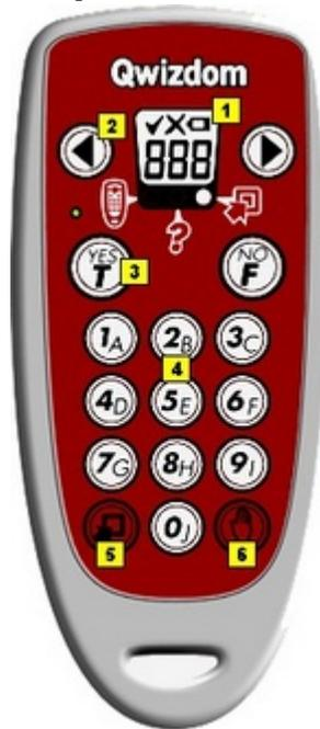
1. E ink™ display-displays the remote's ID number when it is turned off; displays remote's ID number and battery icon when it is turned on.
